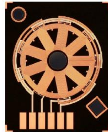
Fig. 1. Axial flux micro-motor: schematic (above) and stator picture
